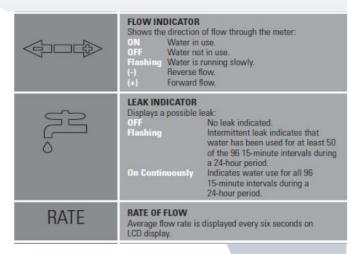
The Aclara STAR system transmits usage and other data, via Data Collector Units throughout the water system, back to our office. This is done nightly, so we are able to get closer to "real-time" information on the water system. The meters can be programmed to read more frequently when needed in determining specific leak information. Graphs and precise daily usage are just a few of the reports that make this system a great customer service tool, while helping the company to track water usage.
